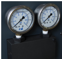
Front Vise pressure regulation for optimal clamping grip
